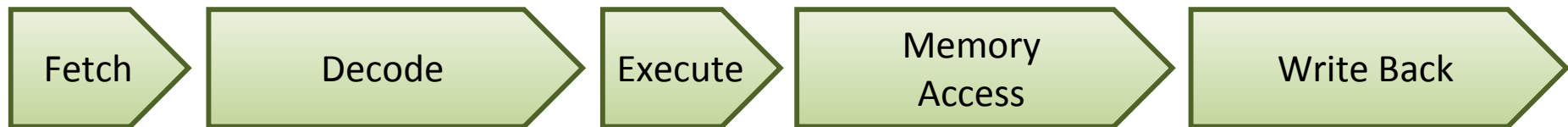
Typical 5-stage Pipeline
