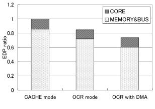
Figure 4. EDP Ratio of SH-4 with DMA
