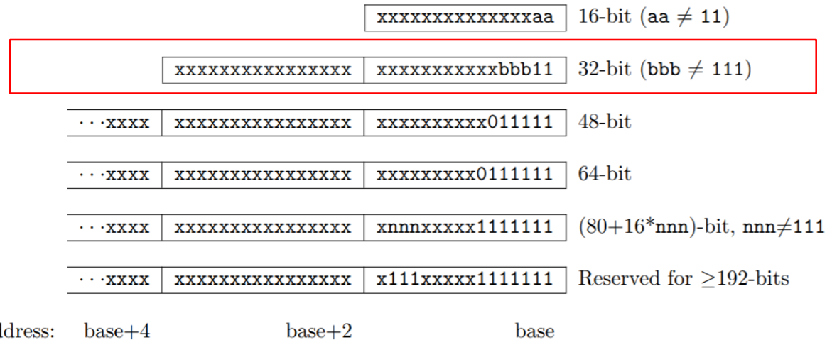
Figure 1.1: RISC-V instruction length encoding. Only the 16-bit and 32-bit encodings are considered frozen at this time.
