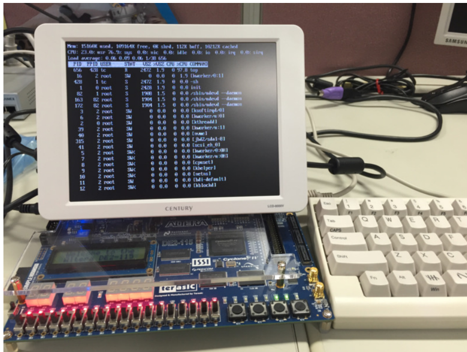
Figure 4.9: The snapshot of Linux (Tiny Core) running “top” command on DE2-115 FPGA board
