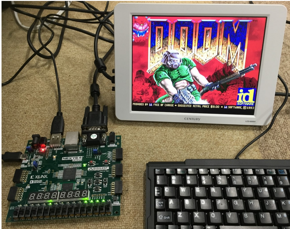
Figure 4.6: The snapshot of DOOM running on Nexys4 DDR FPGA board
